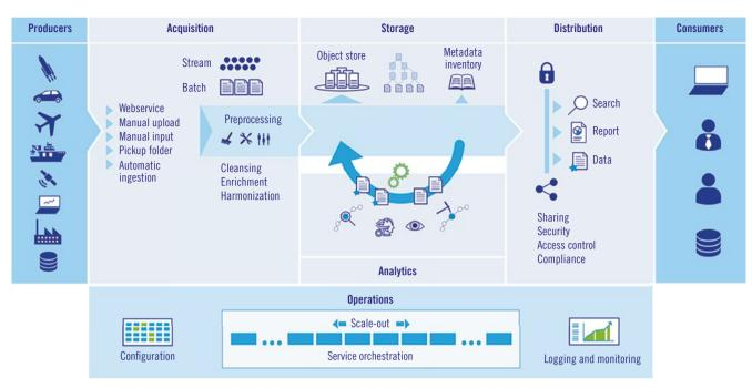
FIGURE 2 Function-oriented structure of a toolchain (© Werum)
